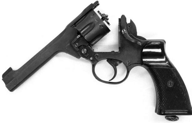
Figure 4.5 The name Enfield is not singular to the bolt-action rifle. Pictured is an Enfield Number 2, Mark 1 revolver chambered in .38/200 British Service. This is a break-top revolver, the lever to open the action is on the left side of the frame adjacent the hammer. Note the spring-loaded ejector, which opens automatically when the action is opened. (Image from author's collection.)
